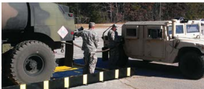
Fail-Safe® MilBerm™ safely captures leaks or spills during refueling operations.
