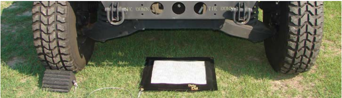
Position drip berm in tight spaces between machinery to capture oily leaks.
