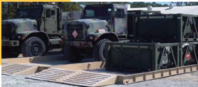
Steel Rigid Containment System for long term containment of fuel trucks and pods.
