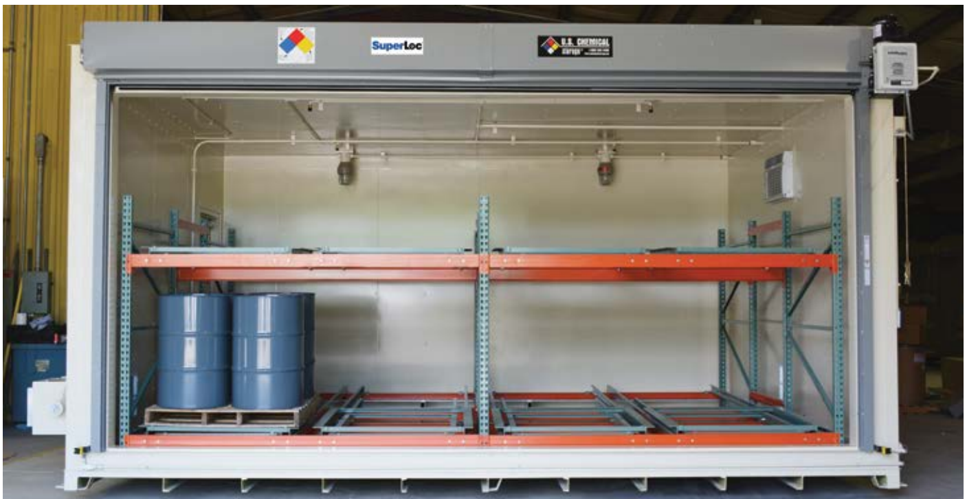
Four-hour fire-rated, 64-drum, SUPERloc™ chemical storage building with explosion-proof (EP) lighting, EP mechanical ventilation, and push-back racking.
