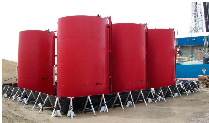
High-wall berm provides secondary containment for horizontally- or vertically-stored metal or poly tanks.
