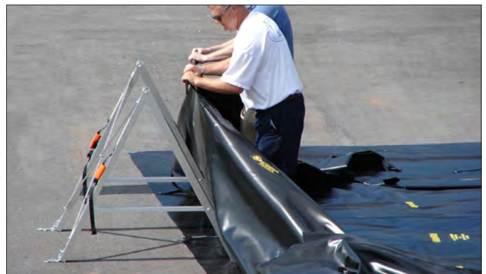
No tools needed to assemble. Securely attach liner portion of the berm to the aluminum A-frame supports which are spaced four feet apart.
