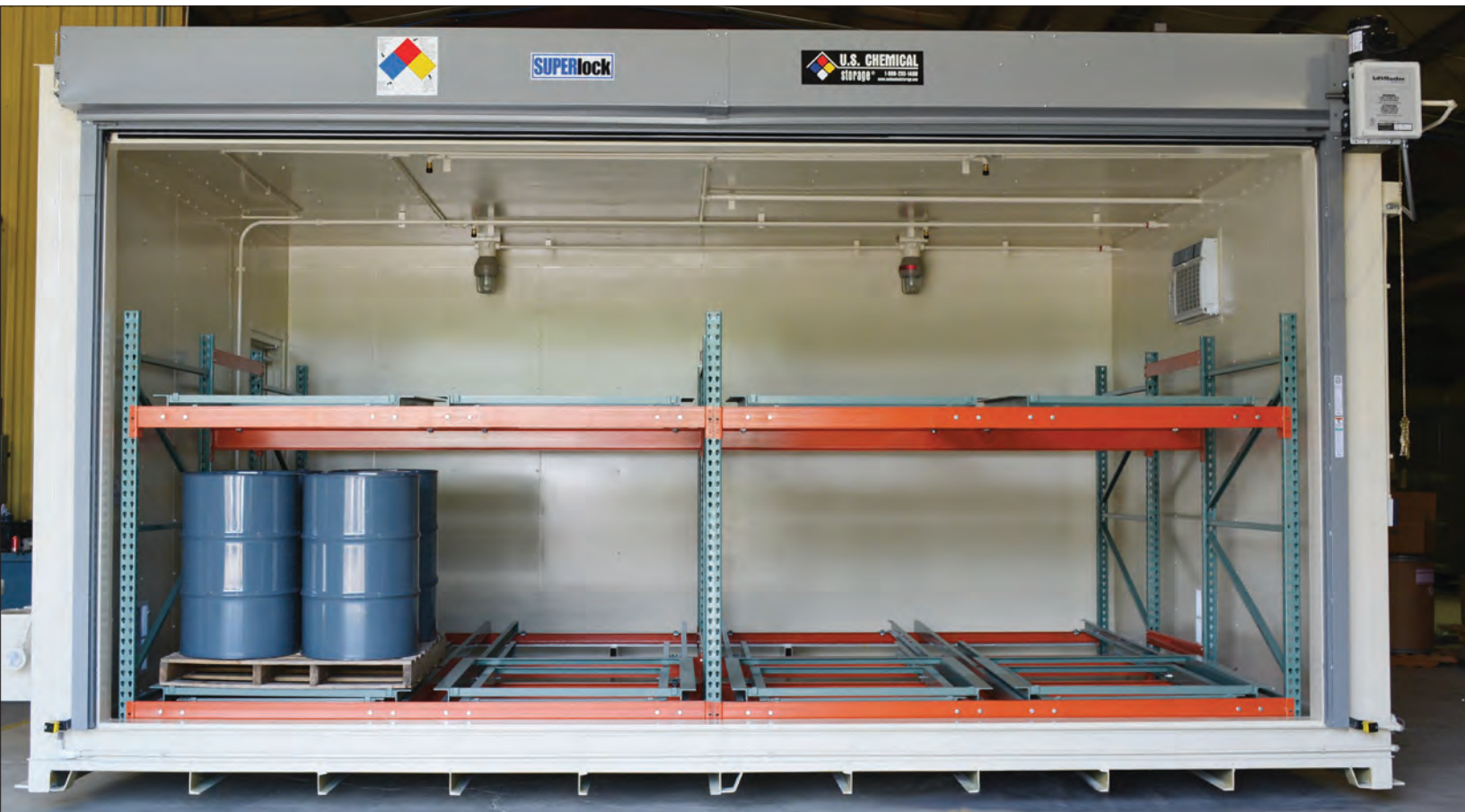
Four-hour fire-rated, 64-drum, SUPERloc™ chemical storage building with explosion-proof (EP) lighting, EP mechanical ventilation, and push-back racking.
