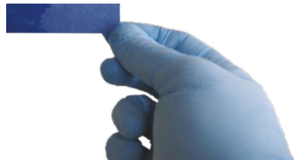
The Hydrocarbon Detection Strip turns a darker blue when hydrocarbons are present.
